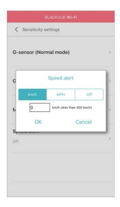
Set a speed limit (up to 300 km/h or 200 MPH) for the speed alert. When the vehicle exceeds the specified speed limit, the dashcam beeps and switches to event recording. After saving one event recording file the dashcam switches back to normal mode recording.
